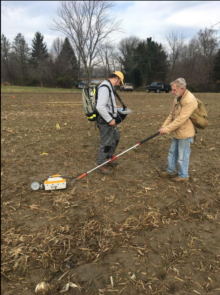
Above: Ground-penetrating radar surveys being undertaken at the Brotherton site.
